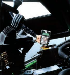
Perfect interaction between hydrostatic transmission, engine and hydraulics: the performance of the truck can be modified to match the requirements of the operator. Automatic engine accelleration on lifting is standard.
