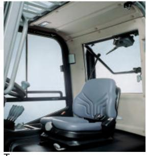
he new full cab, available as an optional, is installed inside the profile of the overhead guard. It is equipped, in the standard version, with high-quality panelling, accessories and soundproofing, lexan roof complete with gutters, sliding windows and pantograph windscreen-wiper for more effective cleaning.
